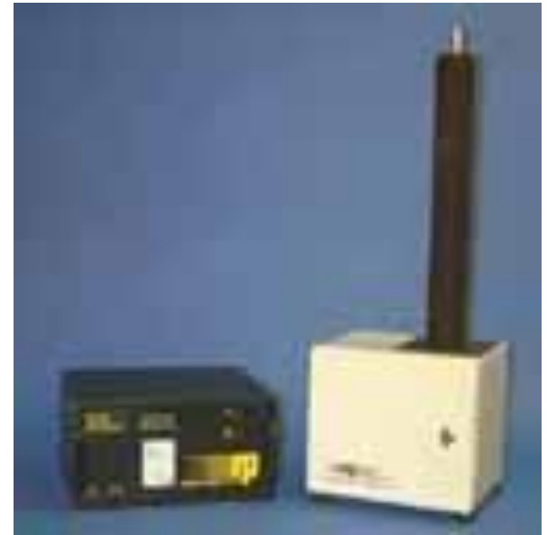
TEOM Series 1400ab Ambient Particulate Monitor Thermo Electron Co.
