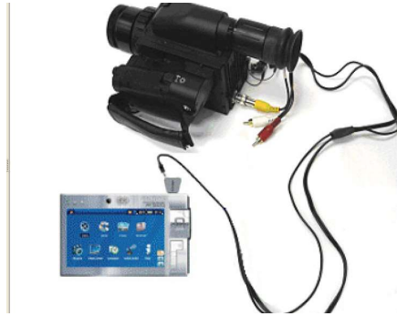
GasFindIR Camera with Digital Recorder (Older Model)
