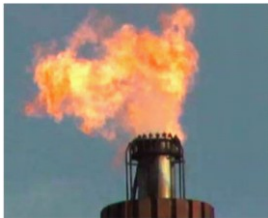
Well Operating Flare - High Combustion Efficiency
