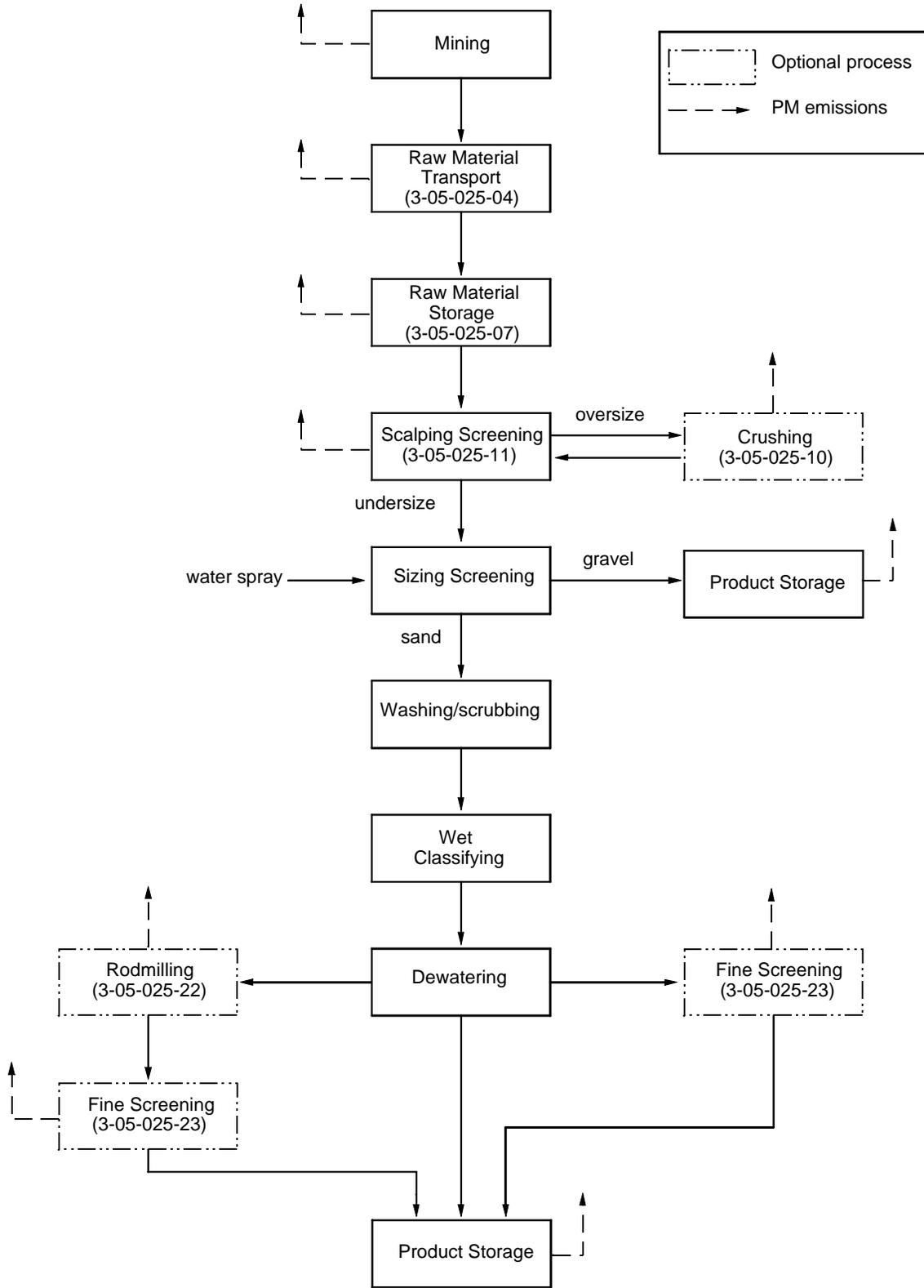
Figure 11.19.1-1. Process flow diagram for construction sand and gravel processing.
