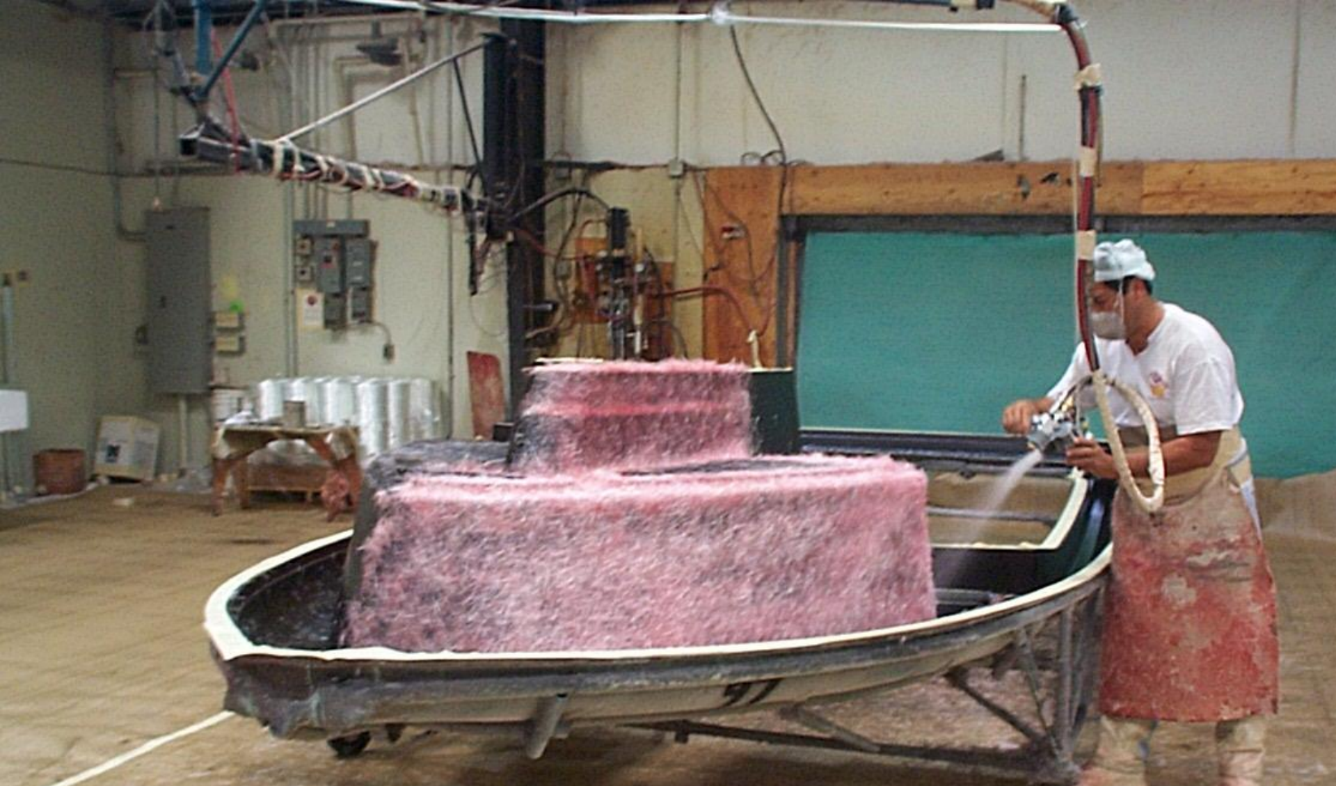
Chopped Fiberglass Spray-up Operation
