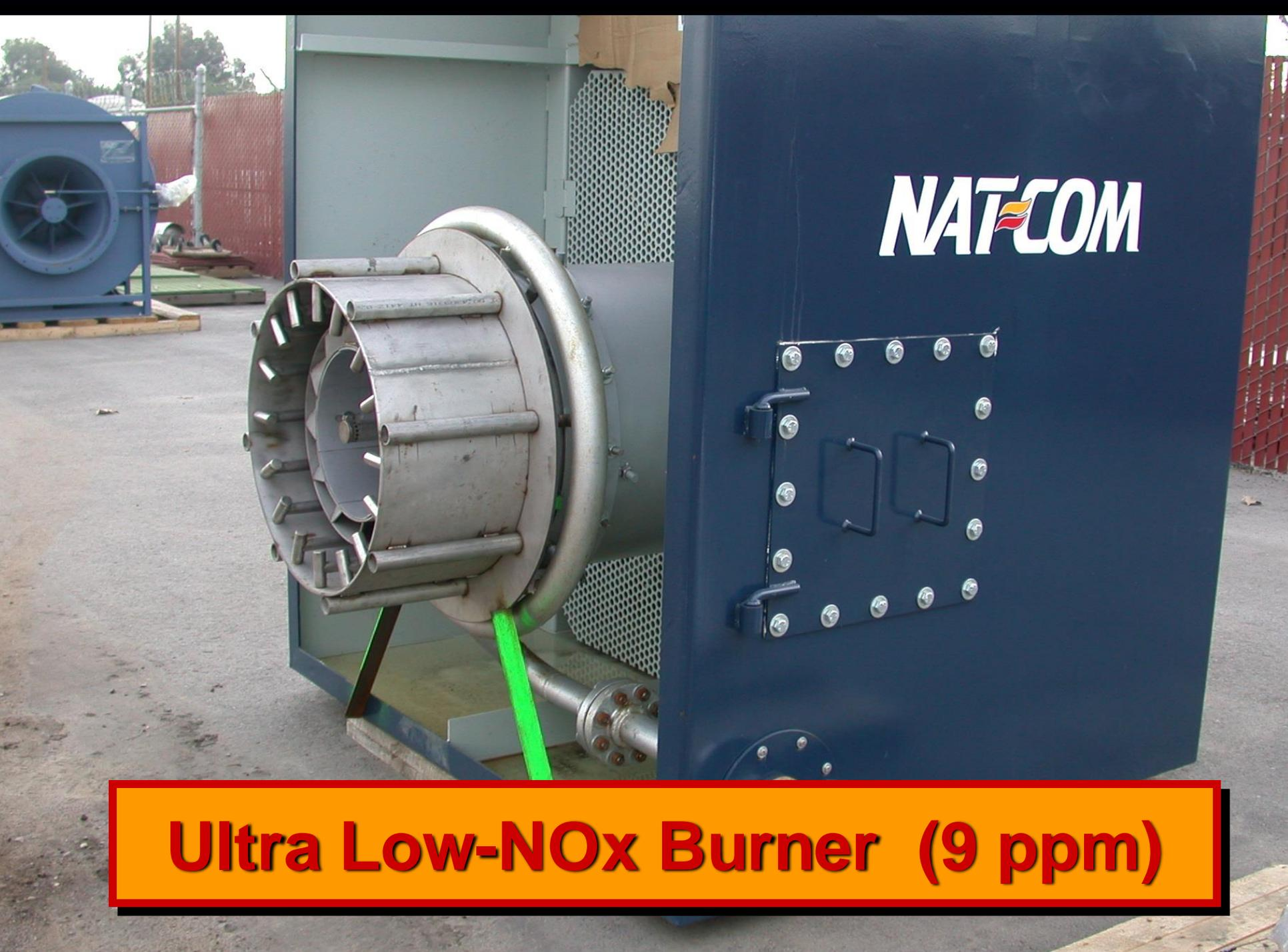
A photograph of a large industrial burner assembly. The burner is a cylindrical metal component with a flange and several horizontal support tubes. It is mounted on a blue metal frame. A bright green gas line is connected to the bottom of the burner. The blue frame has the "NATCOM" logo in white, stylized letters with a red and yellow flame icon. The burner is set against a background of a red metal fence and a blue industrial fan.
