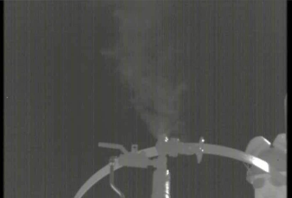
New “alternative work practice” promulgated to allow the use of optical gas imaging as a replacement for method 21
