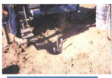
Installation of a Three Tier Probe
